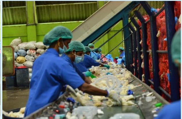
Segregatio of the bio-medical waste after autoclaving
