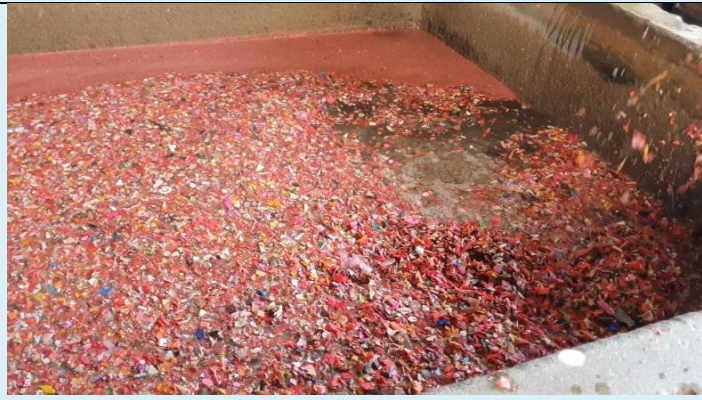
Shredded plastics being washed before turning into pellets
