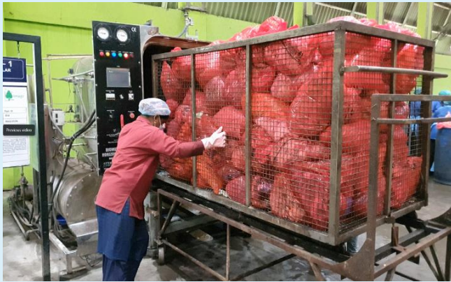
The first step of red category of bio-medical waste is autoclave
