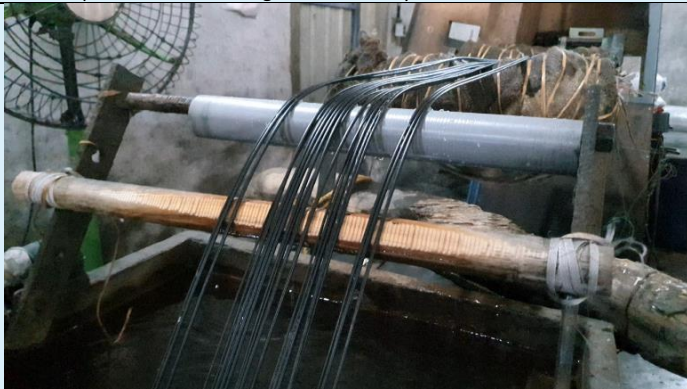
Shredded plastics strings under the process of making plastic granules
